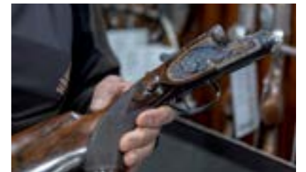
The open-radius semi-pistol-type grip is perfect for the single trigger on this AYA
